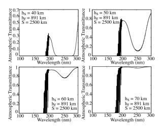
Figure 3. Atmospheric transmittance for four different observation geometries.
