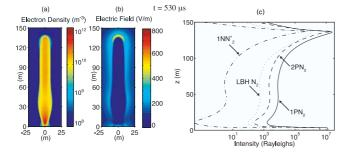
**Figure 1.** Modeling results on a streamer advancing in a weak electric field at 70 km altitude: (a) electron number density, (b) electric field, and (c) intensity (in Rayleighs) profiles of  $1PN_2$ ,  $2PN_2$ ,  $1NN_2^+$  and LBH N<sub>2</sub> emissions along the central axis of the modeled streamer.
