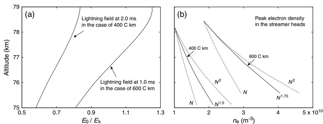
**Figure 4.** (a) Spatial variation of the electric fields induced by the two model lightning discharges, at the moments after the streamers have been initiated. (b) Variations of the peak electron density in the heads of modeled downward propagating sprite streamers shown in Figure 3.
