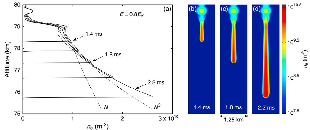
**Figure 1.** (a) Electron density on the axis of symmetry of the downward positive streamer produced by a constant reduced electric field  $E/E_k = 0.8$ . (b–d) Cross-sectional view of electron density of the same streamer at different moments of time.
