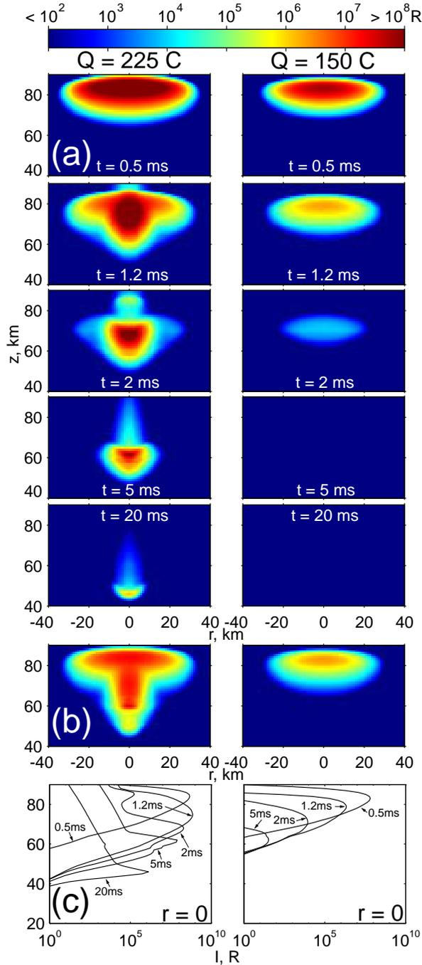
**Figure 2.** The 2D structure of the intensity of the  $N_2$  first positive band at different instants of time after the beginning of the discharge, in Rayleighs,  $Q = 225$  C (left) and  $Q = 150$  C (right),  $\tau_s = 1$  ms: (a) at different instants of time; (b) integrated over 16 ms (approximately one frame of a videocamera); (c) on the axis.
