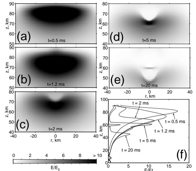
**Figure 3.** The ratio of the electric field to the runaway threshold field  $\delta = E/E_t$  at different moments after the beginning of the discharge ( $Q = 225$  C,  $\tau_s = 1$  ms): (a)  $t = 0.5$  ms; (b)  $t = 1.2$  ms; (c)  $t = 2$  ms; (d)  $t = 5$  ms; (e)  $t = 20$  ms; (f) on the axis.
