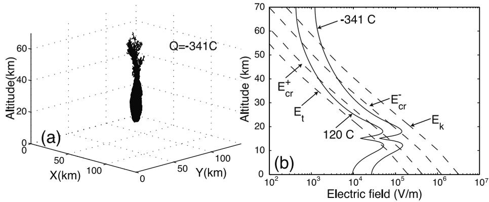
**Figure 11.** (a) Result of the model calculation of a blue jet created by a negative charge  $Q = -341$  C. (b) Altitude scan of the electrostatic fields created by thundercloud charges of 120 and  $-341$  C through the simulation box center (solid lines) along with the characteristic fields  $E_t$ ,  $E_{cr}^+$ ,  $E_{cr}^-$ , and  $E_k$  (dashed lines).
