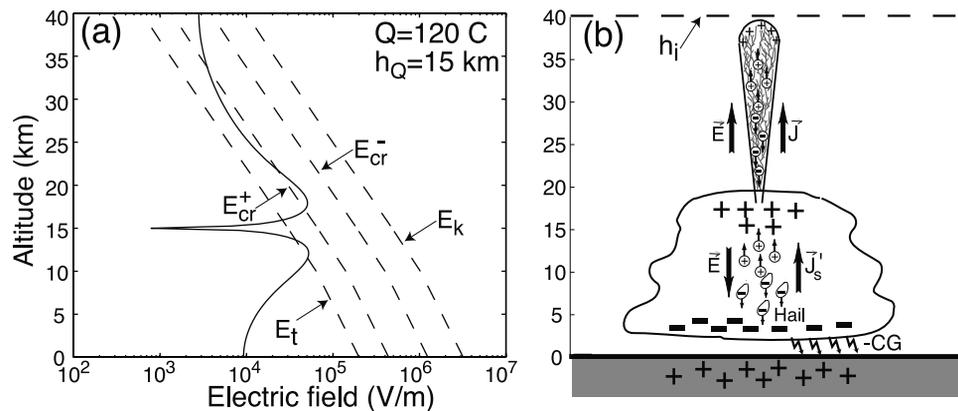
**Figure 1.** (a) Altitude scan of the electrostatic field produced by a 120 C thundercloud charge placed in the center of the simulation box at altitude 15 km (solid line). Dashed lines show the characteristic fields  $E_t$ ,  $E_{cr}^+$ ,  $E_{cr}^-$ , and  $E_k$ . (b) Currents, charges, and electric fields associated with blue jets.
