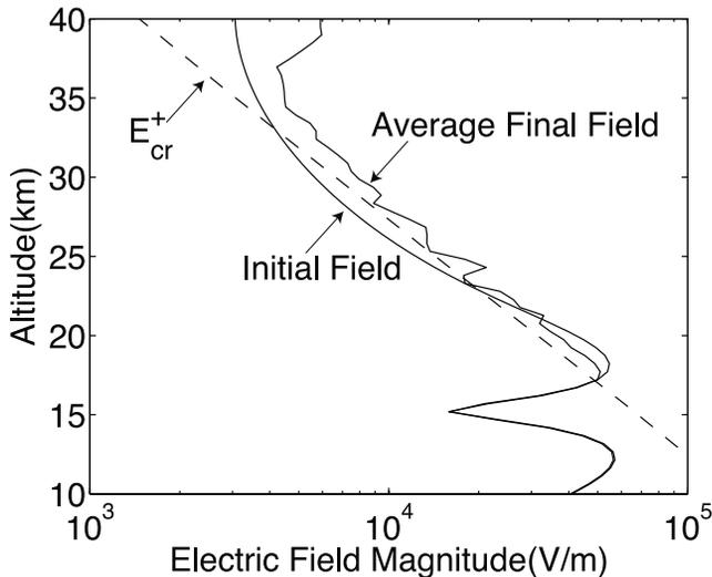
**Figure 5.** Altitude scan of the macroscopic electric fields associated with a blue jet created by a source charge  $Q = 130$  C. The initial static electric field is shown along with the final field after blue jet formation (averaged over 10 blue jet simulations). The critical field  $E_{cr}^+$  is shown, with a dashed line, for comparison.
