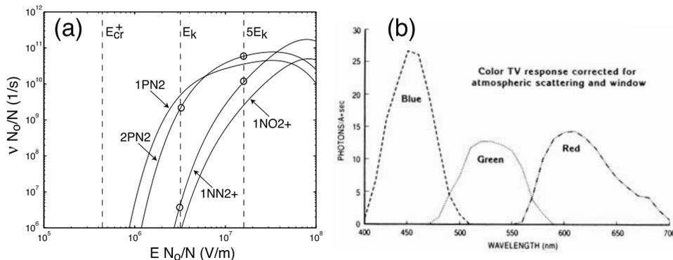
**Figure 3.** (a) Optical excitation coefficients as a function of the reduced electric field in air. (b) Color TV response corrected for atmospheric scattering and transmission through the aircraft window. Figure 3b reprinted from *Wescott et al.* [1998], with permission from Elsevier Science.
