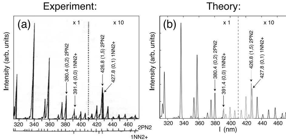
**Figure 6.** (a) Experimental spectrum of the second positive  $N_2$  and first negative  $N_2^+$  bands [Teich, 1993]. (b) Model spectrum corresponding to the same two emissions.
