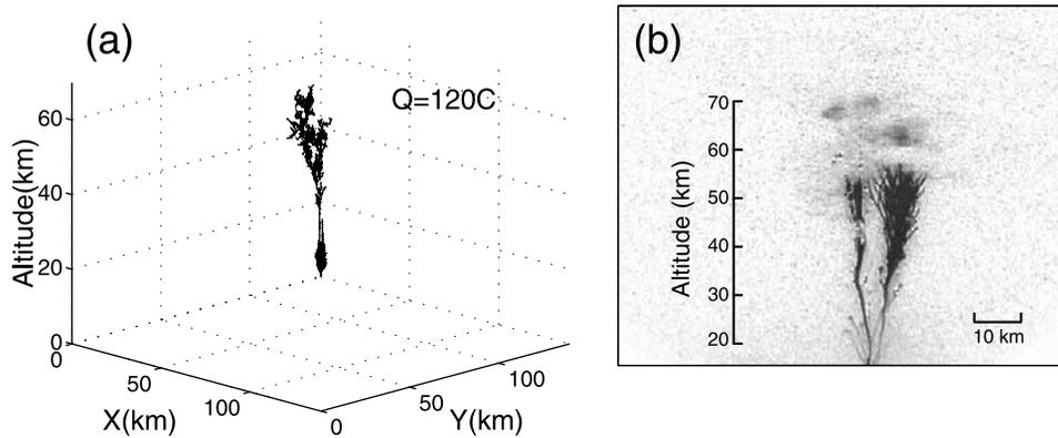
**Figure 8.** (a) Model results for thundercloud charge  $Q = 120\text{ C}$  and the upper simulation box boundary at 70 km. (b) Image of a blue jet at the moment of attachment to the lower ionospheric boundary. Figure 8b reprinted by permission from *Nature* [Pasko *et al.*, 2002] MacMillan Publishers Ltd.
