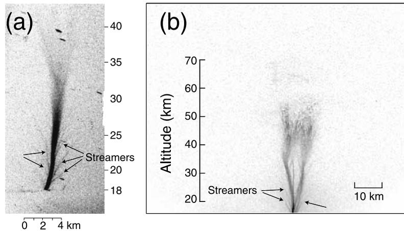
**Figure 10.** (a) A black and white image of a 2-min time exposure of a blue jet. The image is provided through the courtesy of G. Wescott, University of Alaska [Wescott *et al.*, 2001]. (b) Processed image obtained by averaging the sequence of video fields from the study of Pasko *et al.* [2002].
