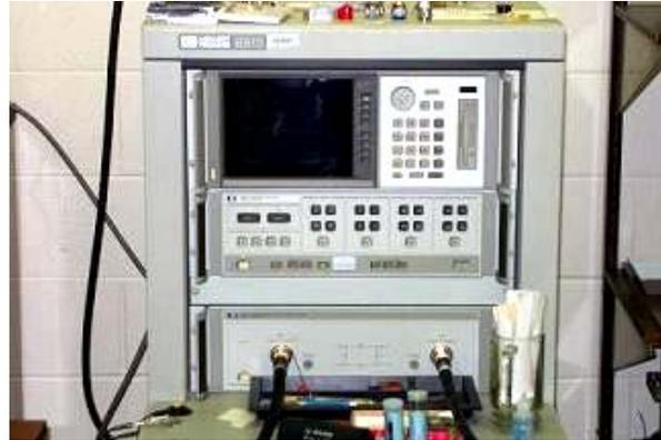
The fixture that was used while electromagnetic energy was sent through the ring resonators was a universal substrate test fixture manufactured by Inter-Continental Microwave, figure III.F.2. This fixture is capable of testing substrates from 0.24 to 4.75 inches long and up to 75 mils thick. In order to calibrate this fixture before use, the TRL-304D Substrate (Alumina) calibration kit was used.
