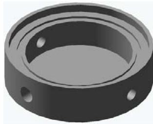
Figure 5: Isometric view of the new vacuum chamber
