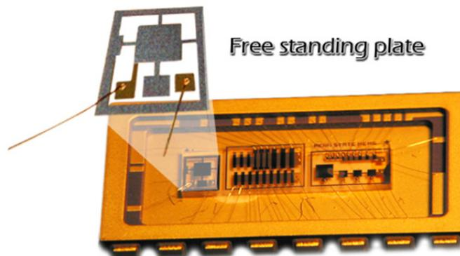
**Figure 2:** Photograph of packaged device and zoomed photograph of Free Standing Plate
