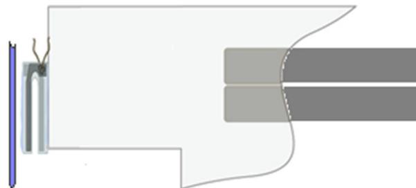
**Figure 3:** Gluing the tuning fork and fiber tip to make a tip and tuning fork holder, reproduced based on reference [7].
