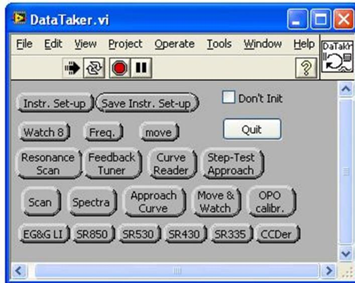
**Figure 4:** DataTaker panel to communicate with the NSOM via the connector box and PCI Data Acquisition (DAQ) card [6].
