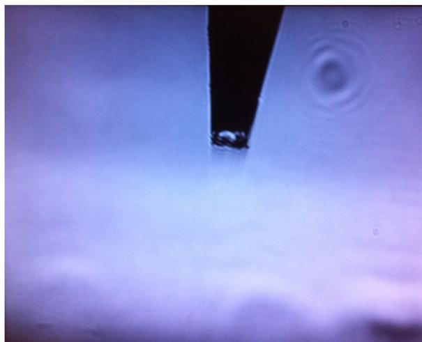
**Figure 7:** The optical fiber tip, coated with aluminum.
