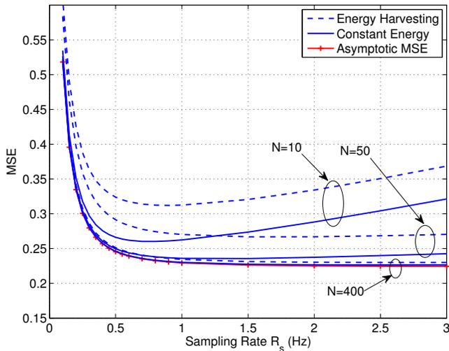
Fig. 2. MSE as a function of the sampling frequency ( $\rho = 0.9$ ).
