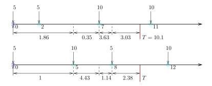
Figure 7.11: Optimal transmit powers  $\mathbf{p}_1 = [1.86, 0.35, 3.63, 3.03] \text{ mW}$ ,  $\mathbf{p}_2 = [1, 4.43, 1.14, 2.38] \text{ mW}$ , with durations  $\mathbf{l} = [5, 2, 1, 2.1] \text{ s.}$
