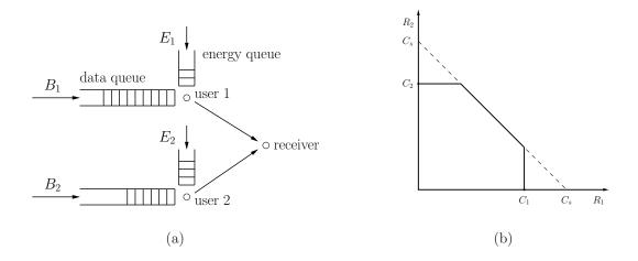
Figure 7.1: (a) An energy harvesting MAC model with energy and data queues, and (b) the capacity region of the additive white Gaussian noise MAC.
