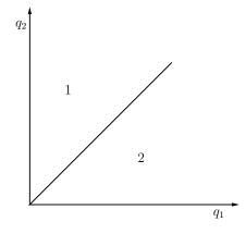
Figure 4.4: The switch structure for a symmetric Gaussian MAC.
