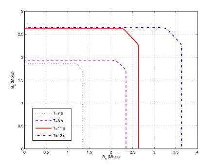
Figure 7.8: The maximum departure region of the multiple access channel for various T.
