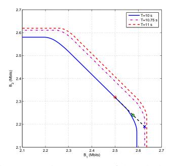
Figure 7.12: The maximum departure region of the multiple access channel for various T.
